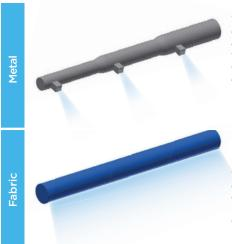
Traditional metal ductwork is heavy, rigid and can only disperse air through spaced out diffusers restricting airflow to localized areas.
